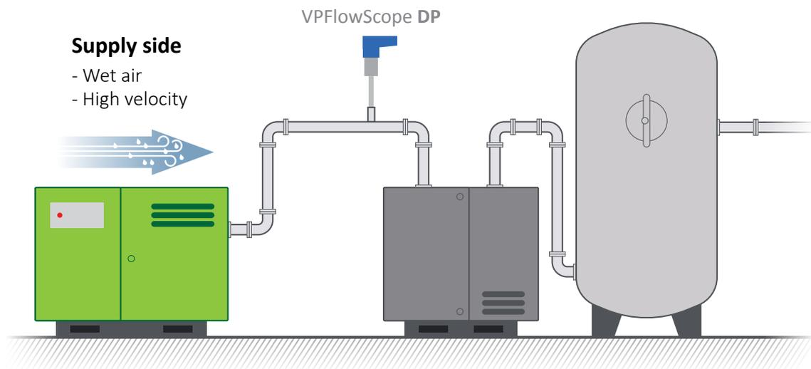
*The VPFlowScope DP is preferably installed in the second horizontal piping after the compressor where there is less possibility for excess water. A cyclone separator is recommended upstream of the flow meter, to remove excess water from the system.*
